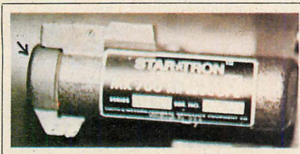
Entire power source for Starlight-type units is normally located on telescope itself. This device uses two 1.35-volt mercury batteries housed in small compartment on right side of scope.
